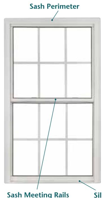
Air Leakage (AL) Rating pertains to the air infiltration that occurs through the window unit itself. It is expressed as the equivalent cubic feet of air passing through a square foot of window area per minute. For example, the sash meeting rails, sash perimeter and sill are typical areas where air leakage may occur. Poorly designed windows do not have the necessary barriers to block air from forcing its way in and can be a substantial source of energy loss in a home.
